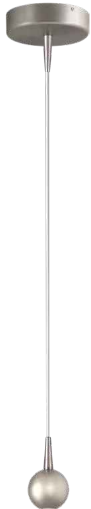
2410-37-37 Nickel Fixt. Nickel Shade, 4,4W 450Lm 3000-2200K, Triac-Dim.
